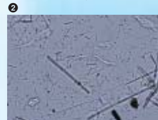
Chrysotile and amosite (refraction index of the liquid n 0 = 1.605, 40x objective)
