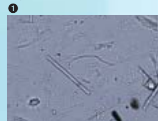
Chrysotile and amosite (refraction index of the liquid n 0 = 1.605, 40x objective)
