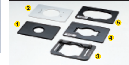
AZ-STD Diascopic Stand, AZ-STGD DIA Stage, AZ-SG Stage Glass
