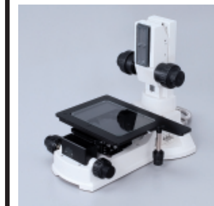
AZ-STD Diascopic Stand, AZ-STGD DIA Stage, AZ-SG Stage Glass
