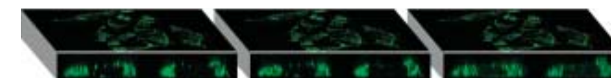
PFS on: 41 sequential XZ sectional images taken by changing the Z-axis position. Almost no photobleaching occurred thanks to a reduction in scans.
