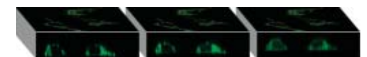
PFS off: 65 sequential XZ sectional images taken by changing the Z-axis position. 24 extra pictures were taken to cover focus drift. Strong photobleaching occurred due to frequent scans.
