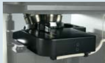
Perfect Focus System with motorized sextuple DIC nosepiece (Ti-E)
