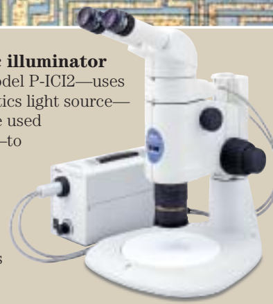
SMZ1500 configured with the coaxial episcopic illuminator
