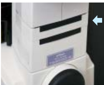
Eye-level riser (as indicated by arrow)
