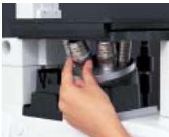
Nosepiece is inclined to the left for easy handling.
