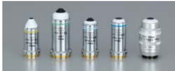
CFI Plan Fluor 10x W, NA 0.3, W.D. 3.5mm CFI75 LWD 16x W, NA 0.8, W.D. 3.0mm CFI Apo 40x W NIR, NA 0.8, W.D. 3.5mm CFI Apo 60x W NIR, NA 1.0, W.D. 2.8mm CFI Plan 100x W, NA 1.1, W.D. 2.5mm
