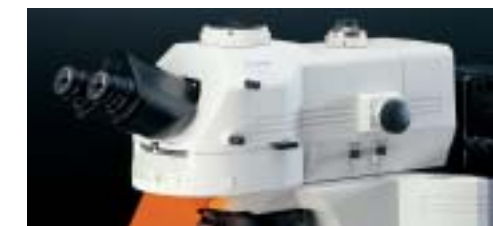
DIH-M: Manual model (only epi-fl shutter motorized)
