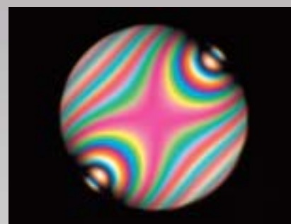
Conoscopic image of mica / CFI P Achromat 40X
