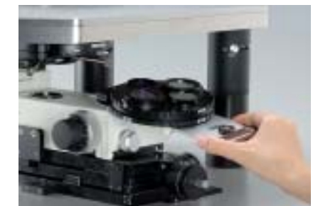
The condenser and polarizer turret can be simply and quickly removed.
