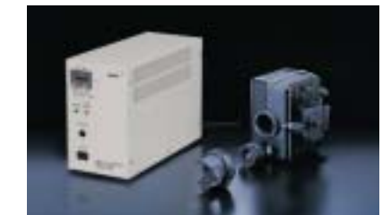
Mercury lamphouse for episcopic illumination
